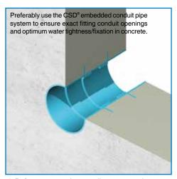
1) Before starting the installation procedure, any dirt or concrete residues should be removed from the conduit inlet pipe.
