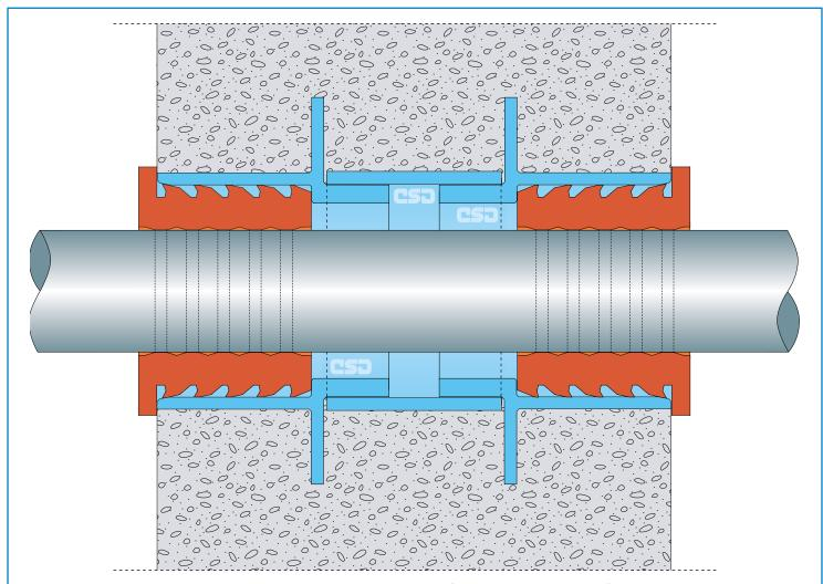
Optimized gas and water tightness is obtained by applying the SLIPSIL® sealing plugs in the CSD® embedded conduit inlet system or in the CSD® flanged conduit sleeves. These offer optimum ease of installation, prevent any damage to the plugs during insertion and prevent the plugs from being inserted too deep into the conduit opening. The sealing plugs also can be used in holes bored with diamond-tipped drills. The tolerances of the drilled hole should be within the tolerances of the plug series.
