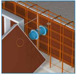
6) The formwork element is then removed so that the CSD® fixation piece can be affixed.
