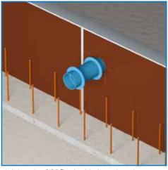
2) Adapt the CSD®embedded conduit inlet system to the width of the formwork by sawing the CSD® adjustment pipe to length in situ. Press the CSD® conduit inlets and adjustment pipe over the installed fixation piece.
