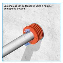
6) Then both segments of the SLIPSIL® sealing plug are pushed by hand evenly, serration by serration, further into the conduit opening.
