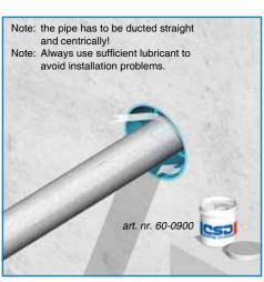
2) The inside wall of the conduit inlet pipe is treated with CSD® lubricant up to the shoulder inside the conduit inlet pipe. In case of non-CSD® conduit sleeves, sharp edges have to be rounded off to avoid damage to the plugs.
