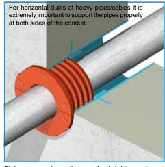
9) In cases where the required tightness is not excessive, a SLIPSIL® sealing plug can be installed at one side of the conduit. Only applicable in combination with CSD® embedded conduit pipe system.
