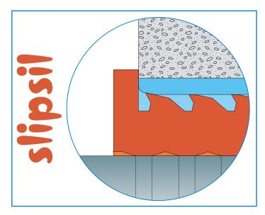
With the application of the CSD® embedded conduit inlet system in combination with the SLIPSIL® sealing plugs, not only the installation of the sealing plugs is extremely simple and effective, but leakages via conduits in new installations is prevented. The systems can be used for conduits through which cables, metallic or plastic pipes are ducted. Durability guaranteed: the SLIPSIL® sealing plugs do not age and are UV. Ozone and weathering resistant.
