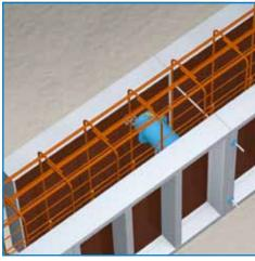
5) The formwork element is provisionally positioned so that the position of the CSD® fixation piece to be fitted can be marked off.
