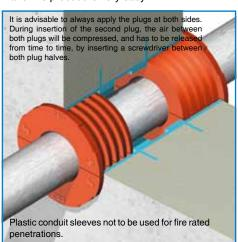
8) SLIPSIL® sealing plugs always have to be inserted in both ends of conduits for heavy pipes, when to cope with settling in front of the foundation, in drilled holes and for fire rated penetrations.
