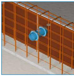
3) For very wide formwork, two or more CSD® adjustment pipes are used. The adjustment pipes are linked with the aid of CSD® connectors.
