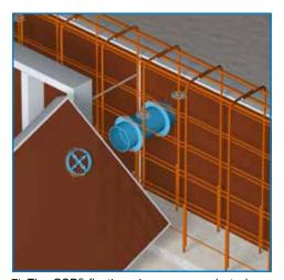
7) The CSD® fixation pieces are made to be a clamping fit for fixation in the CSD® conduit inlets for reasons of stability but also to prevent concrete running into the conduit inlets.
