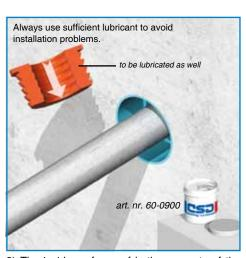
3) The inside surfaces of both segments of the SLIPSIL® sealing plug are then treated with CSD® lubricant. For selecting the right sealing plug, look for the plug series and the plug type in this series on the basis of the ID of the conduit and the OD of the ducted pipe.
