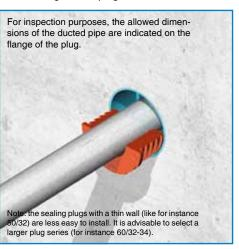
5) Both segments of the SLIPSIL® sealing plug are placed around the ducted pipe and then pushed into the conduit opening as far as the first serration. The first serration is smaller than the other serrations to make this procedure very easy.
