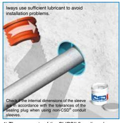
4) The segments of the SLIPSIL® sealing plug are also treated with CSD® lubricant on the outside. Please refer to the Safety Data Sheet of the CSD® lubricant for more information.
