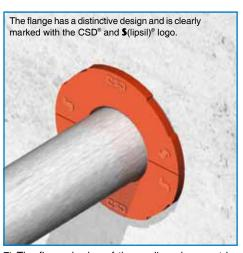
7) The flanged edge of the sealing plug must be flush against the front side of the wall. The shoulder inside the conduit pipe inlet prevents the SLIPSIL® plug from being inserted too deep into the conduit opening.
