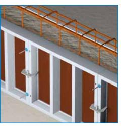
8) The flanges of the CSD® conduit inlets serve for fixation into the concrete and also act as a water barrier. The CSD® embedded conduit inlet system is made of impact-resistant plastic.
